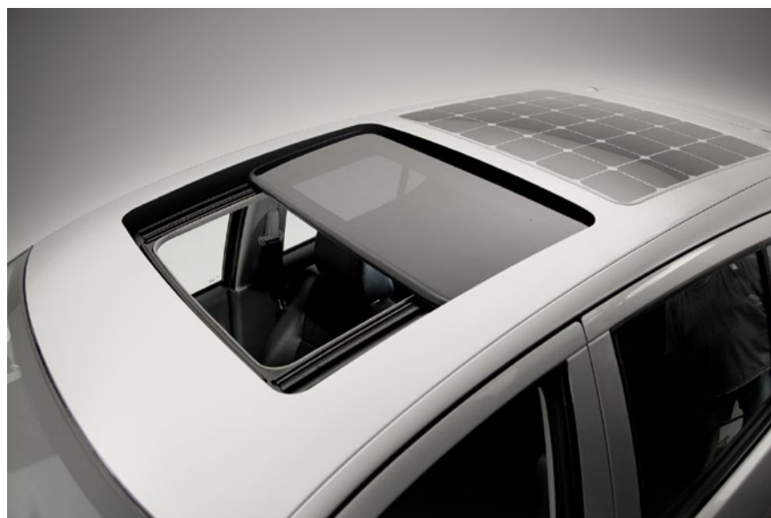
❶ The lightweight design roof module combines comfort with solar power generation
