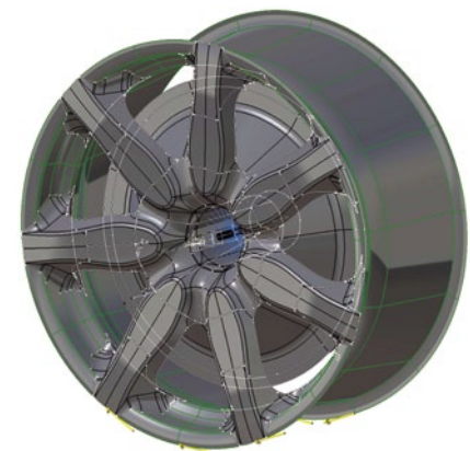
③ Structure of the zones for layer definition, storage conditions and the application of force for the load case "braking"
